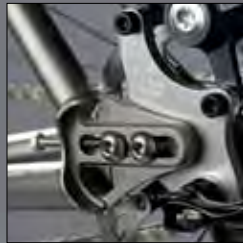
SLIDER DROP OUTS: Lighter, better holding power and easier adjusting than EBB.
