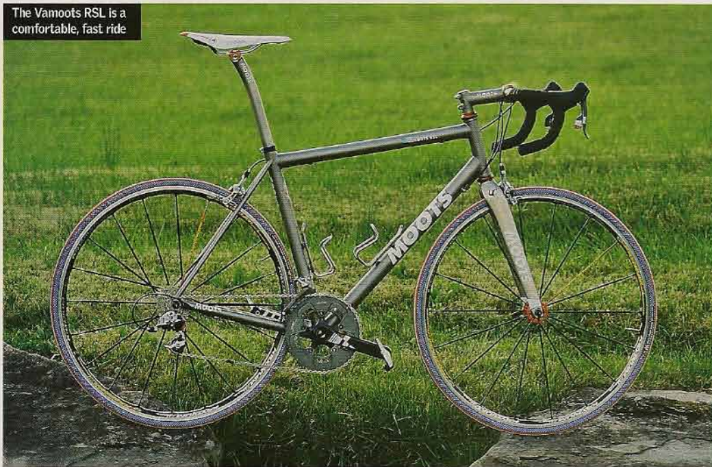
The titanium frame helps iron out vibration
